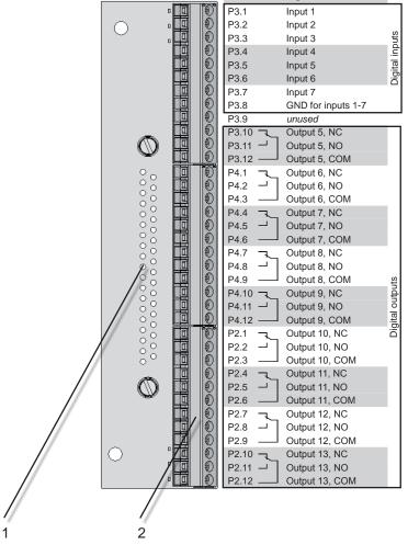
Recommended wire gauge: 0.14...1.5 mm<sup>2</sup>, end sleeves not required
